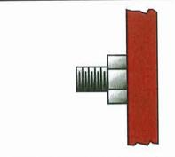
Figure 3. Example of a hazardous projection that extends more than 2 threads beyond the nut and forms an impalement/laceration hazard and may also be an entanglement hazard.
