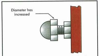
Figure 2. Example of a hazardous projection that increases in diameter from plane of initial surface and forms an entanglement hazard and may also be an impalement hazard.
